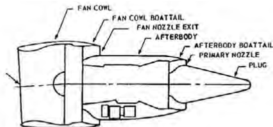
Figure 38.19 - Typical high bypass engine nacelle. Source: AIAA Paper No. 81-1694
