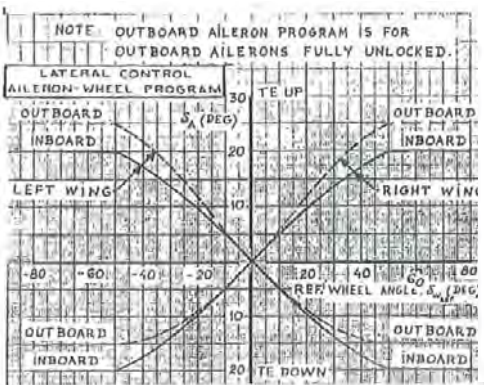
Figure 34.13 - Gearing between control wheel and roll control surfaces - Boeing 747-100. Source: NASA CR-114494
