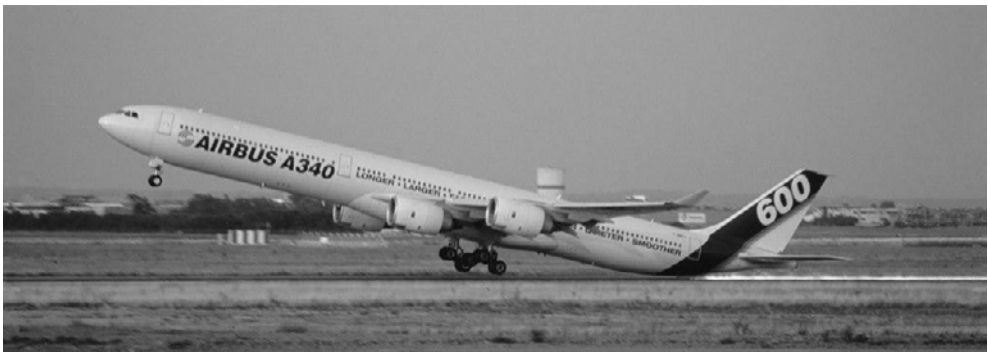
Figure 44.16 - Airbus A340-600 V_{MU} test. Source: Yannick Delamarre
