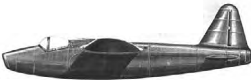
Figure 20.3 - Heinkel 178, the first jet-powered airplane in the world
