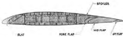
Figure 24.55 - Outer wing section parallel to wing ribs. Source: SAE Paper S408
