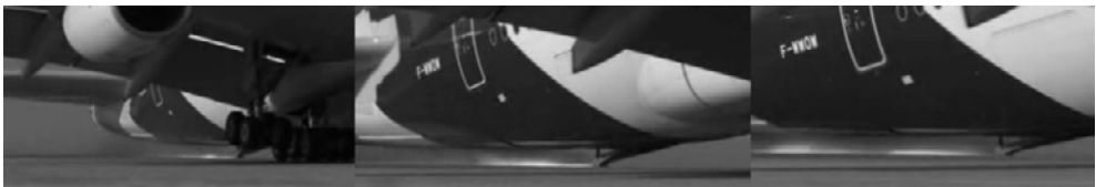
Figure 44.17 - Airbus A380 V_{MU} test. Source: Airbus
