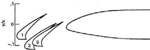
Figure 25.11 - Changing slat position to improve the pressure distribution on an airfoil section with a slat and a flap at \alpha = 15^\circ and \delta_f = 10^\circ . Re = 3.8 \times 10^6 . Source: NASA TM 78566
